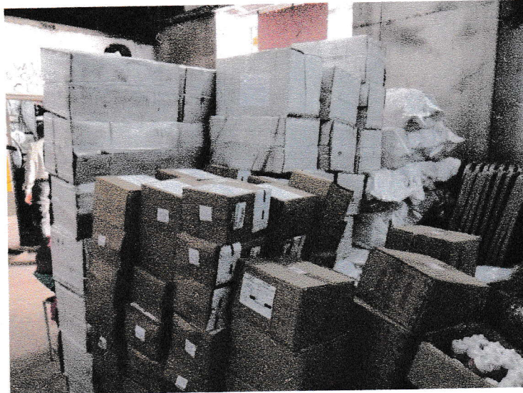
Fig.1: Storage of Elastic ring in main store at CLW (not recommended)
