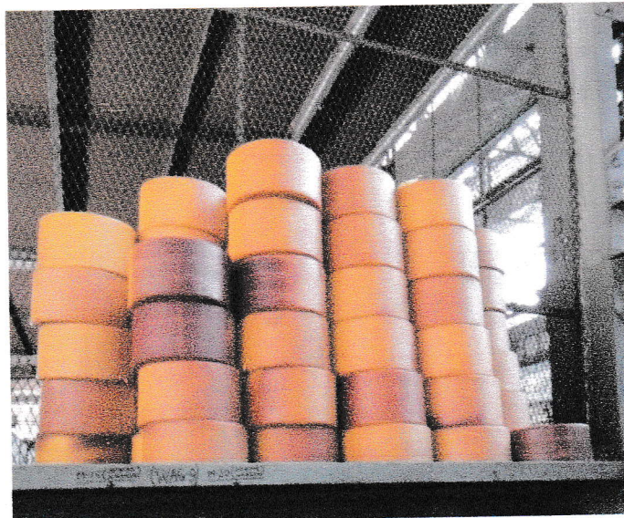
Fig.2: Storage of Elastic ring in shop at CLW (not recommended)
